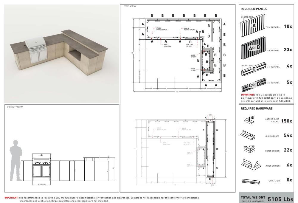
IMPORTANT: It is recommended to follow the BBQ manufacturer's specifications for ventilation and clearances. Belgard is not responsible for the conformity of connections, clearances and ventilation. BBQ, countertop and accessories are not included.
