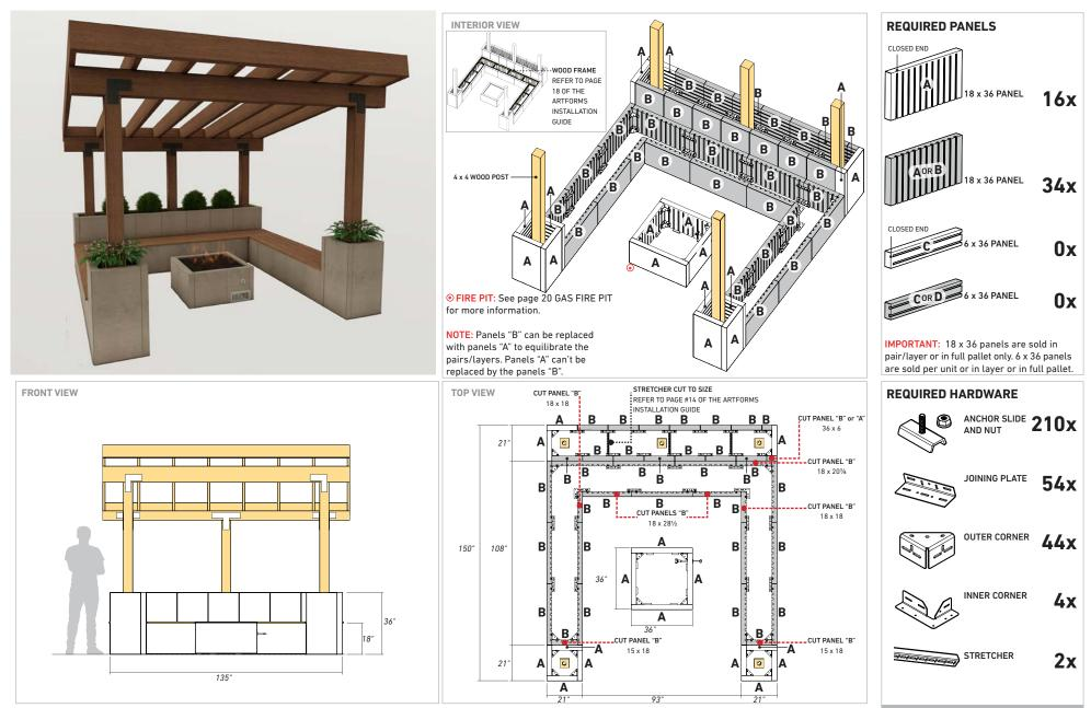
IMPORTANT: Other types of hardware (not included) may be required to make these assemblies (wood screws, concrete anchors, etc.). BELGARD is not responsable for any issue regarding other materials, accessories, other types of hardware, etc. We recommend to consulting an expert/engineer to validate installation of the wood posts of pergola.
