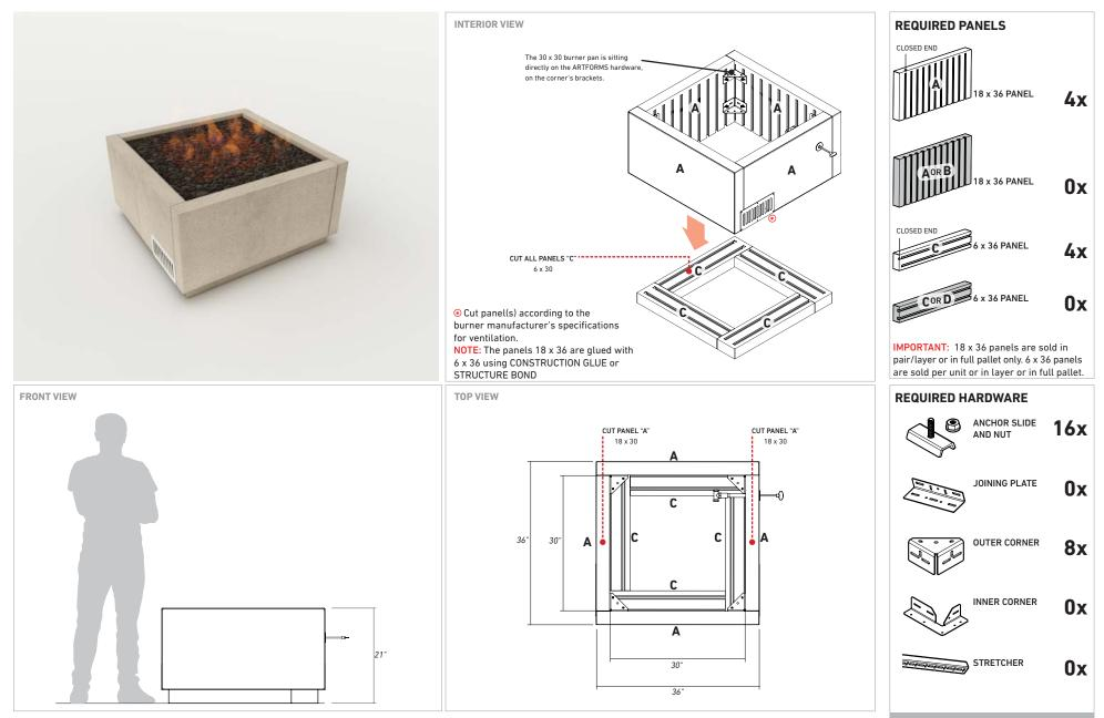
IMPORTANT: It is recommended to follow the burner manufacturer's specifications for ventilation. Belgard is not responsible for the conformity of connections, clearances and ventilation. Burner pan and accessories are not included.
