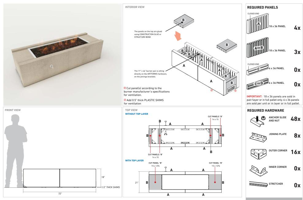
IMPORTANT: It is recommended to follow the firekit manufacturer's specifications for ventilation. Belgard is not responsible for the conformity of connections, clearances and ventilation. Burner plate and accessories are not included.
