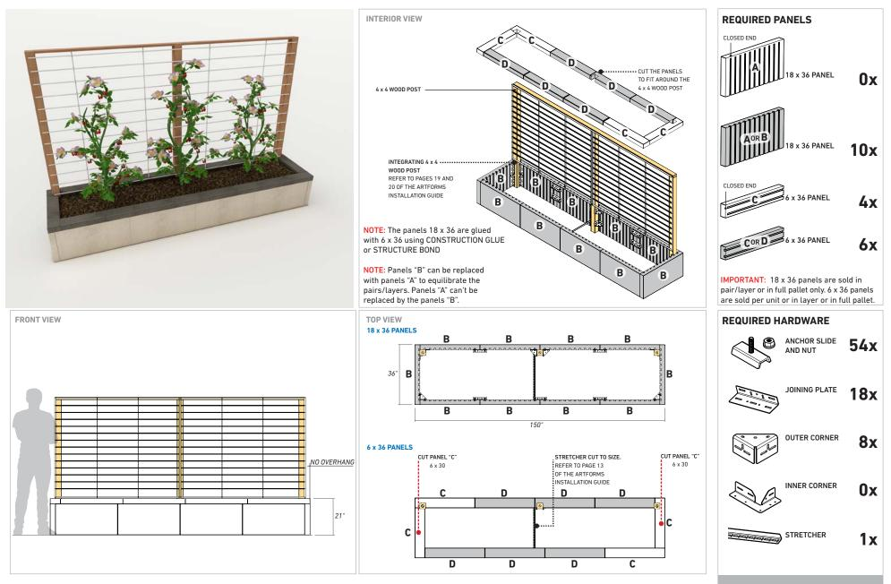
IMPORTANT: Refer to page 23 of the ARTFORMS INSTALLATION GUIDE about the installation of geotextile in planter box. Contact experts/engineers to validate the base preparation, the drainage, the plants & roots growth/management. 1986 Lbs
