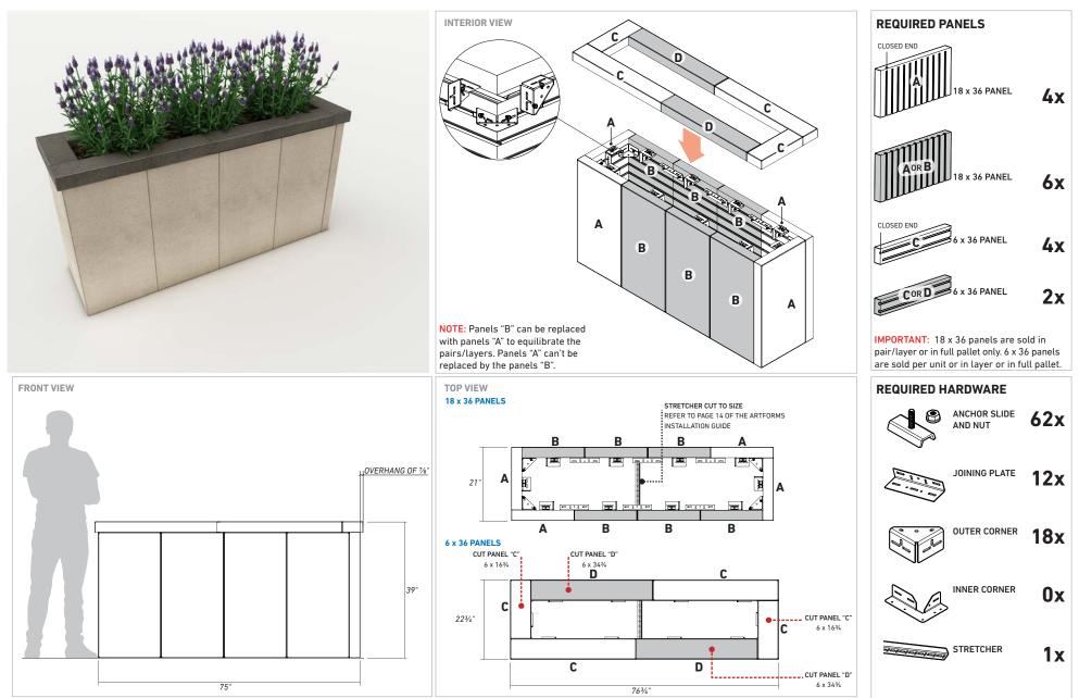
IMPORTANT: Refer to page 23 of the ARTFORMS INSTALLATION GUIDE about the installation of geotextile in planter box. Contact experts/engineers to validate the base preparation, the drainage, the plants & roots growth/management. 1765 Lbs
