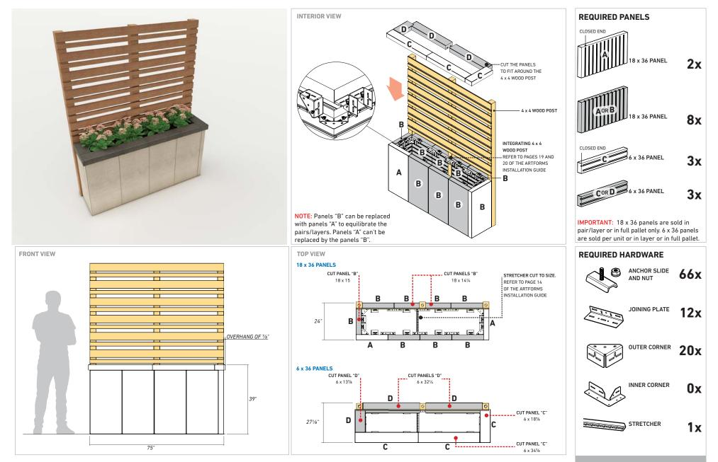
IMPORTANT: Refer to page 23 of the ARTFORMS INSTALLATION GUIDE about the installation of geotextile in planter box. Contact experts/engineers to validate the base preparation, the drainage, the plants & roots growth/management. 1667 Lbs
