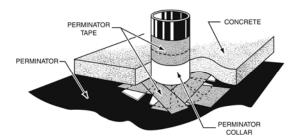
In the event that PERMINATOR is damaged during or after installation, repairs must be made. Cut a piece of the vapor barrier large enough to cover any damage by a minimum overlap of 6" (152.4 mm) in all directions. Clean all adhesion areas of dust, dirt and moisture. Tape down all edges using PERMINATOR TAPE.
