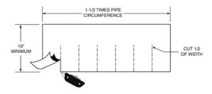
2. Wrap around and tape the collar onto the pipe and completely tape fingers to the bottom layer of PERMINATOR, as shown in figure 2.
