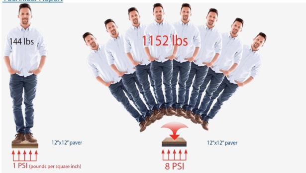
1 PERSON OF 144LBS ON A 12" X 12" PAVER PRODUCES 1 PSI LOAD
