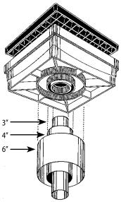
**Choice of 3 drain pipe sizes.** Three bottom drains are molded in. The AD1 can be drained with 3" Schedule 40, 4" SDR35, and 6" ASTM3034 pipe.
