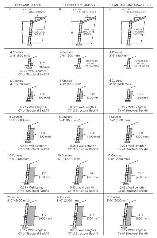
Detail shown is conceptual only and should not be used for construction without the seal of a local qualified engineer.
